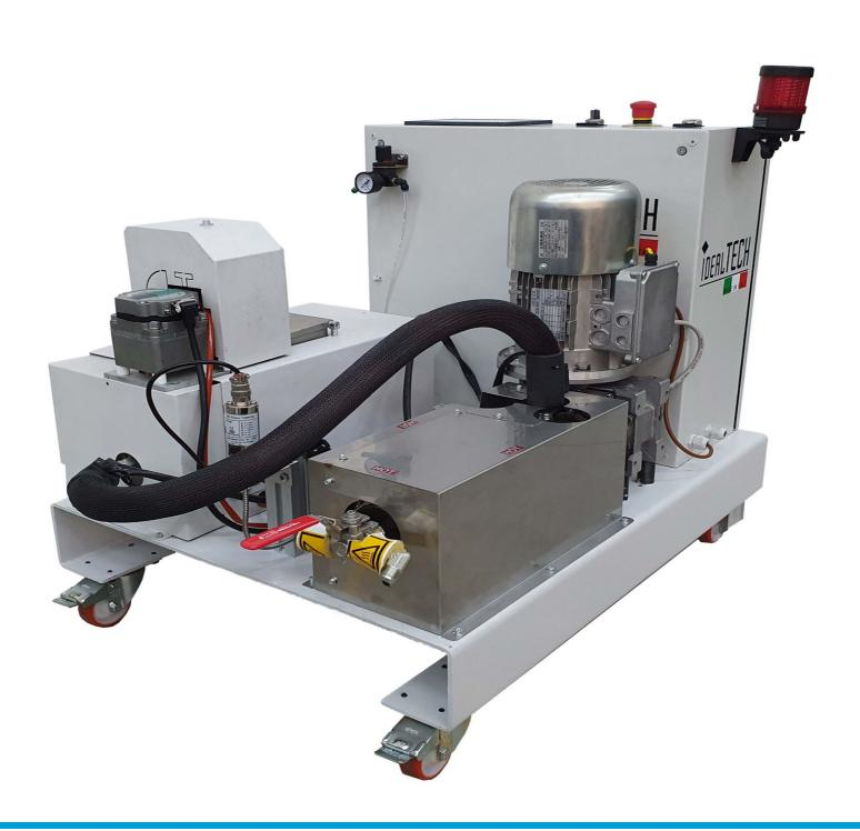
Flat tank melting unit with piston pump doble effect has a 4 kg capacity tank completely covered with Teflon. It is equipped with the following accessories:
